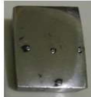
Speciment after Hardness Test
