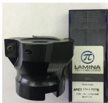
*Figure 3. Milling head and inserts*
