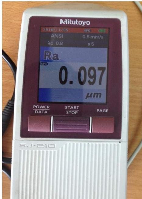
Figure 4.SJ-210 Mitutoyo for surface roughness
