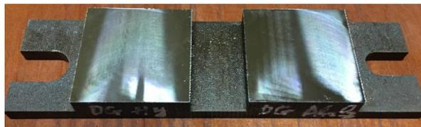
*Figure 2. Hardox 500 steel workpiece*
