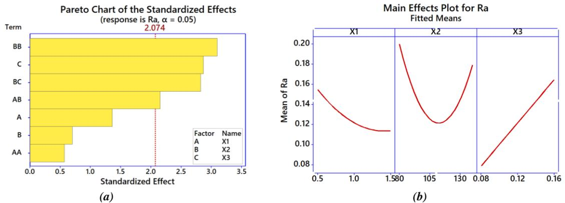
Figure 5. Pareto chart of the effects of investigated parameters on surface roughness  $R_a$ : (a) Pareto chart, (b) Plot of main effects
