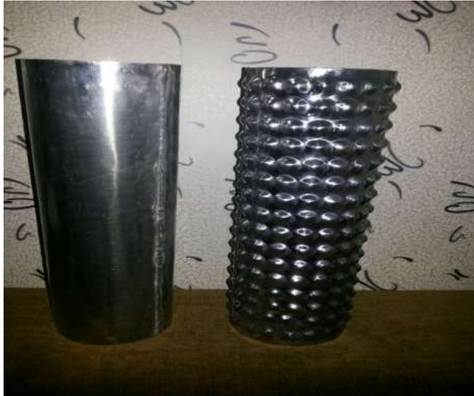
Figure 4.31 Plain and Modified body of silencer
