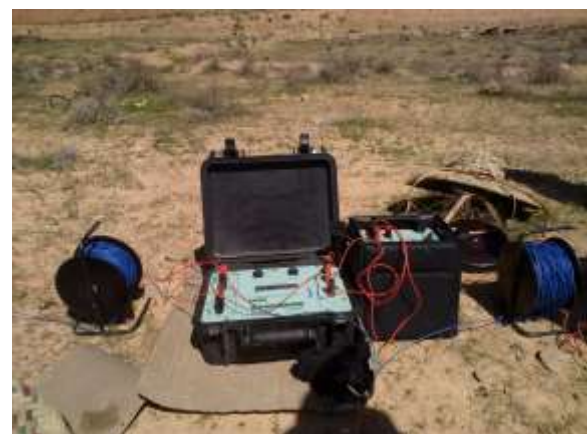
Figure 3: it indicates the geophysical device PASI whose model is 16GL. Contribute a better translation.
