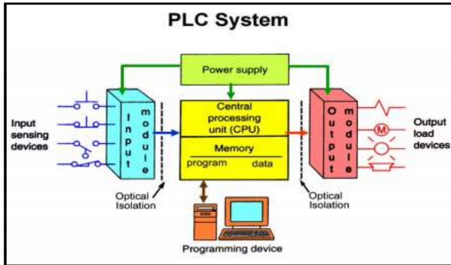
Fig. 2: (a) Block Diagram of Programmable Logic Controller
