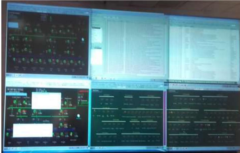
Fig. 3: GUI of SCADA showing substations control parameters in Indore Project work
