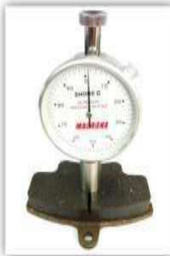
Figure V(a). Hardness Test ( Shore' s D Hardness machine)
