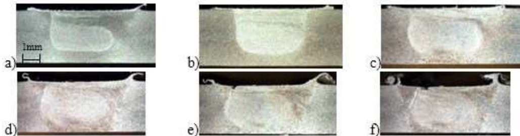
Fig.11 HRS-FSW in 3.2 mm 6061-T6 at a) 3000 rpm, b) 4500 rpm, c) 6000 rpm, d) 7500 rpm, e) 9000 rpm, and f) 12,000 rpm
