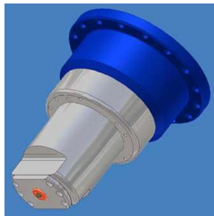
Fig.6 Fixed Shoulder Tool Design
