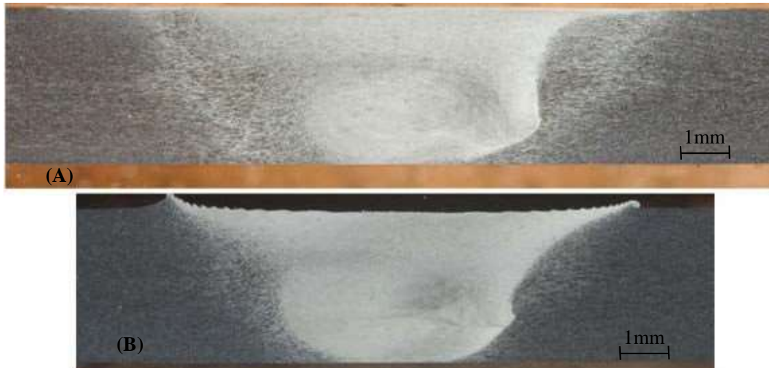
Fig. 9 A Comparison of Weld Macros Using a Conventional Fixed Pin Tool (A) With Fixed Shoulder Tool and (B) Without
