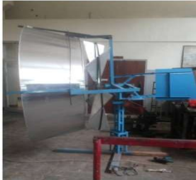
Fig 2.2. Installed wind turbine with cone tunnel
