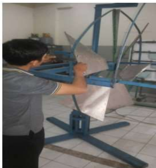
Fig. 2.1. Building and installing wind turbine
