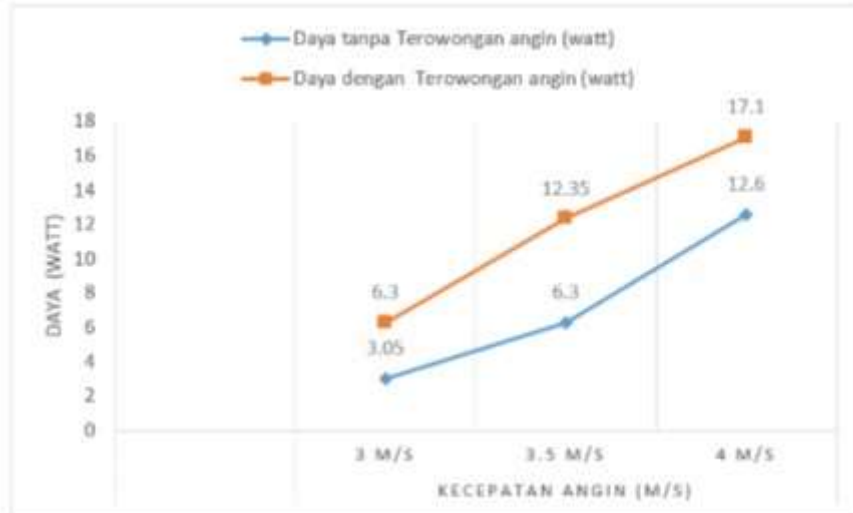
GRAPH 4.1. THE INCREASE OF TURBINE POWER BY USING CONE TUNNEL
