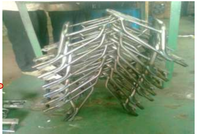
Figure 7 Over loading of material and poor material handling
