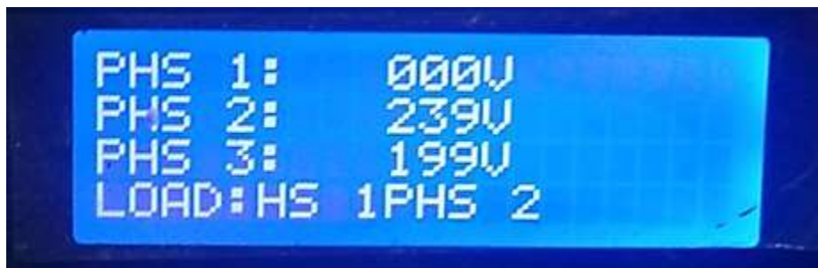
Figure 12.0: Displayed value for logic Output 0 1 1
