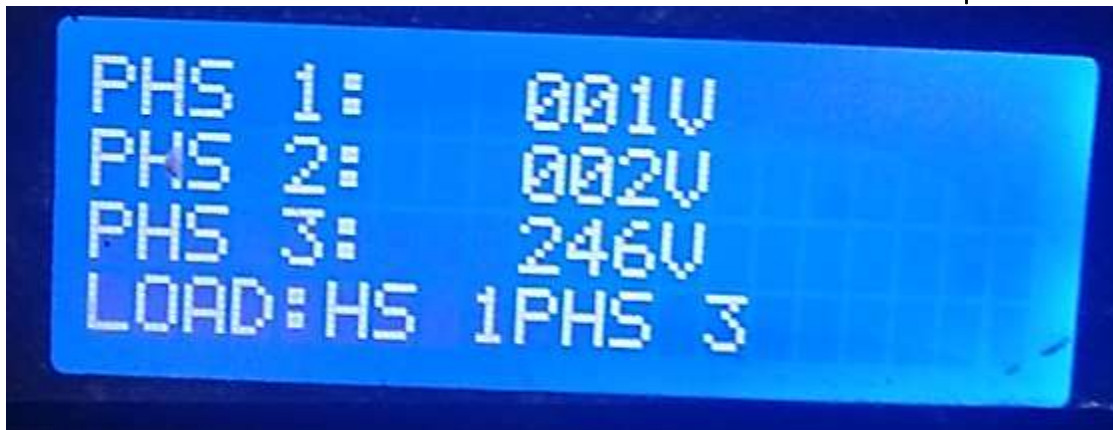
Figure 14.0: Displayed value for logic Output 0 0 1
