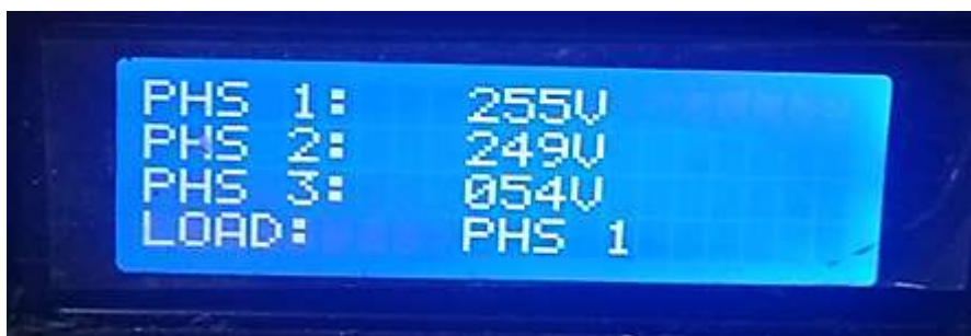
Figure 9.0: Displayed value for logic Output 1 1 0
