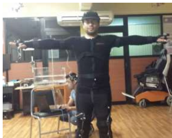
Figure 7. Optimal placement of inertial sensors
