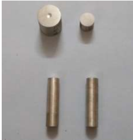
Figure 4. Hardness, Microstructure and Wear Testing Specimens
