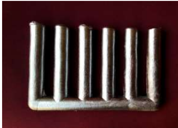
Figure 3. Casted composites of different percentages of Zirconium
