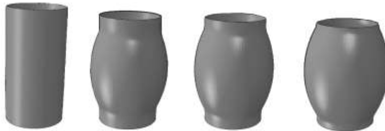
Figure 6. Membrane buckling in numerical modeling
